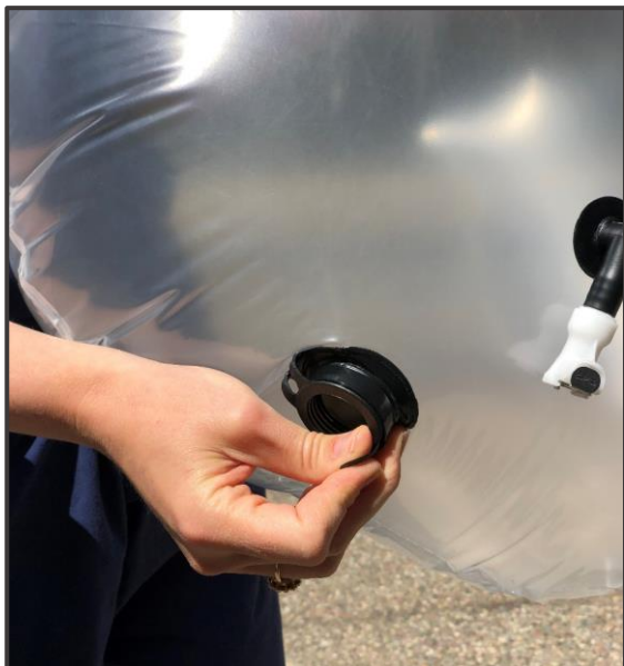
Figure 8. Emptying the Exhaust Collection Bag outdoors
