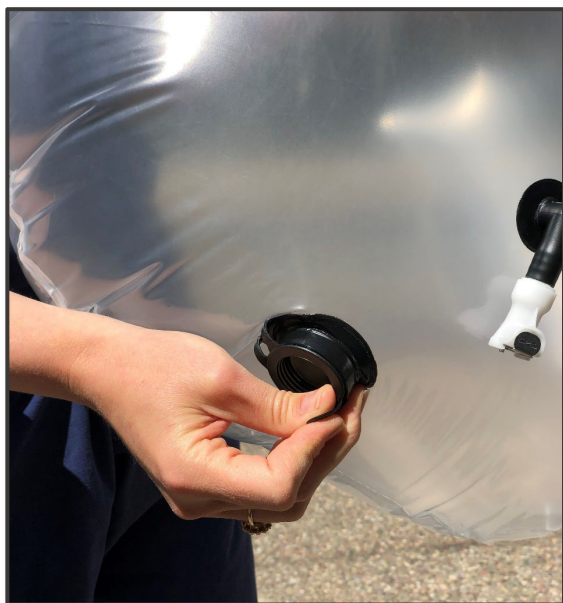
Figure 8. Emptying the Exhaust Collection Bag outdoors
